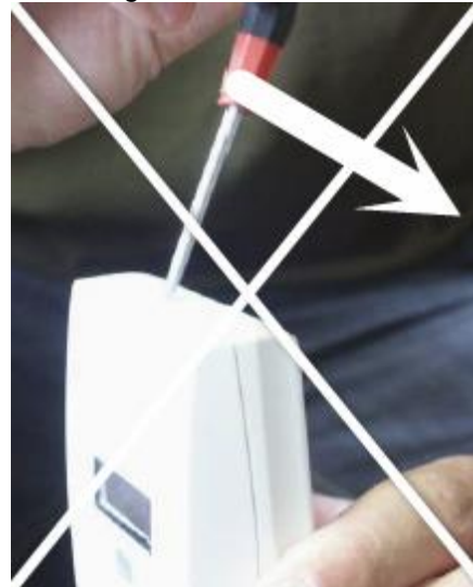
Figure 3. Closed housing seen from the side. Never push to the right. The locking hooks may break and the housing is damaged
